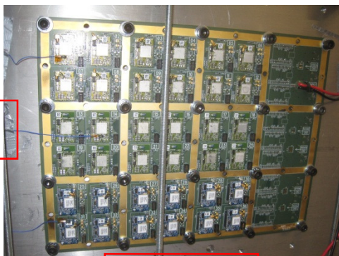
Accelerometers on DUTs
