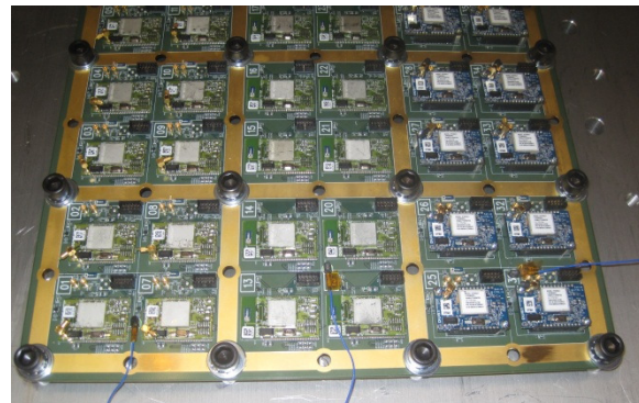
Accelerometers on Board in Proximity to DUTs
